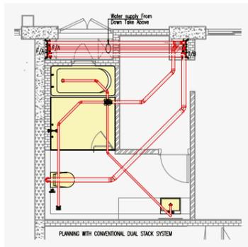
Planning with a conventional drainage and ventilation system
